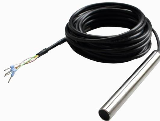
The AquaSense DO-O is an optical sensor type PSt3 and electro-optical module in one probe. The sensor has a maximum measurement range of 0 - 100 % O<sub>2</sub>, and a detection limit of 0.03 % O<sub>2</sub>. These probes are waterproof and can be submerged completely so they are ideally suited for e. g. environmental research applications, aquaculture, and measurements in sewage.
